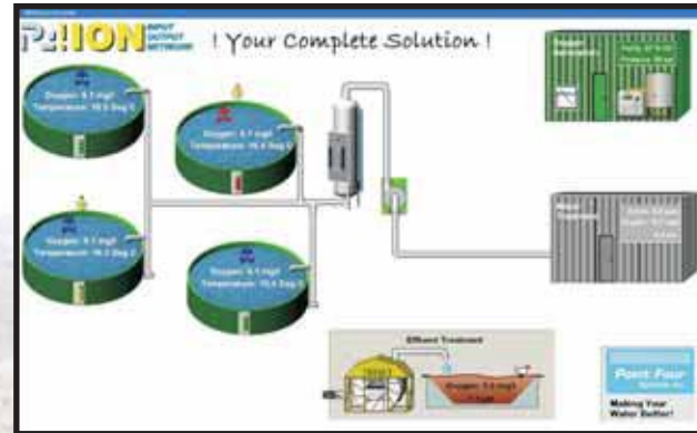
22" LCD Screen Shot - Real-time Water Quality Readings & Trending
